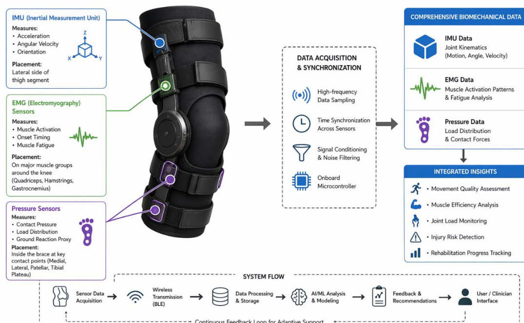
Figure 4: Integration of IMU, EMG, and pressure sensors within the smart knee brace for comprehensive biomechanical data acquisition
